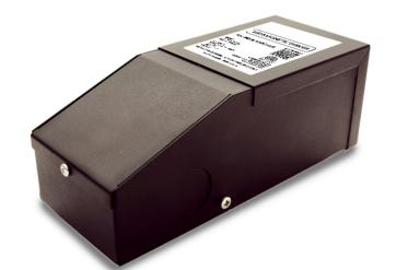
KLUS - MD-100-24 is the most compact LED driver on the market with a magnetic transformer core. It is equipped with two auto-reset breakers, one on the input and one on the output, which protect both the load and driver. The driver is encased in a coated metal box that includes 2 knock-outs, one on each side, to enable easy installation that complies with electrical code requirements.
